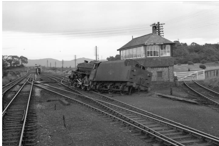
Derailed at catchpoint at Plumpton Junction (showing branch to quarry on right)
